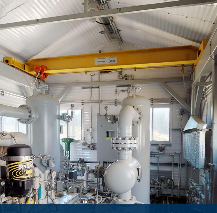
There are three of these units available that are functionally & basically the same, built by Enerflex. Two were built in 2010 & one was in 2012. They were originally built to compress air into an underground formation. They all have Waukesha F18GL LCR drivers and Ariel JGJ/2 compressors. Process can be operated either as a single or a two stage compressor. Control is handled with an Allen-Bradley HMI. All CRN's in this unit are .213 and the vessels/bottles are fully flanged.
